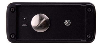
The illustration shows the optional 6pin connector used for digital I/Os
