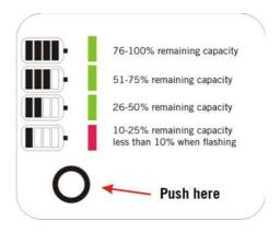
The 205x battery shows the capacity on a front-side display.
