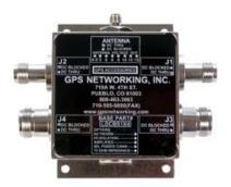
The LDCBS1X4 GPS antenna splitter from GPS Networking, Inc. is a one input four output power divider designed specifically for the GPS L1, L2 & GLONASS carrier frequencies. Three of the output legs (J2-J4) are DC-Blocked to prevent antenna damage; they also have 200 ohm DC loads to ground to simulate a GPS antenna preamp current draw. The other output leg (J1) is a DC through to power the antenna. All GPS Networking GPS antenna splitters are available with N-type, SMA or TNC connectors.
